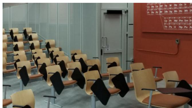
The lecture halls were gutted; removing everything except the casework in the front of the rooms. The single main door and aisle were replaced with two access doors and two aisles. The circa 1939 seats were replaced with a more modern ergonomic style including a foldable tablet-style desk.
